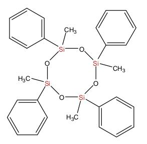
SiSiB® PC9185: Pentamethyl-pentaphenyl-cyclopentasiloxane 10~20%
